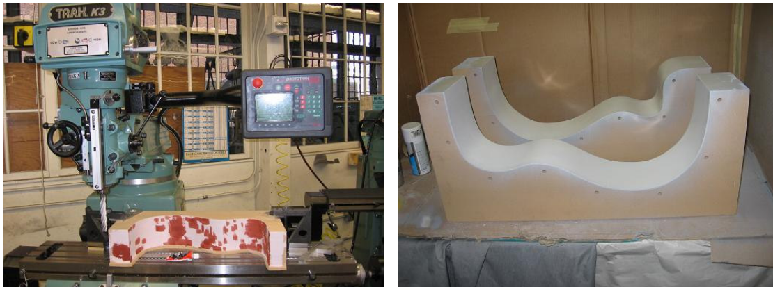
Figure 6.1: Side mold before final machining pass (left), side molds after spray-coating with primer (right)
