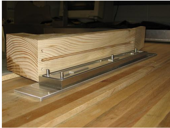
Figure 7.1: Vacuum fixturing for the neck milling
