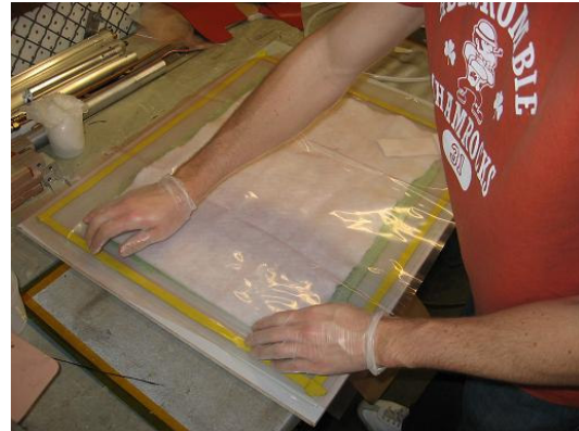
Figure 6.7: Sealing vacuum bag
