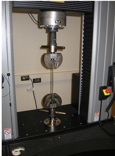
Figure 2.1: Carbon fiber specimen undergoing tensile testing
