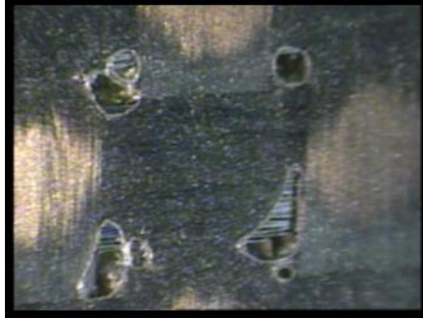
Figure 6.10: Epoxy voids (~40x Mag)
